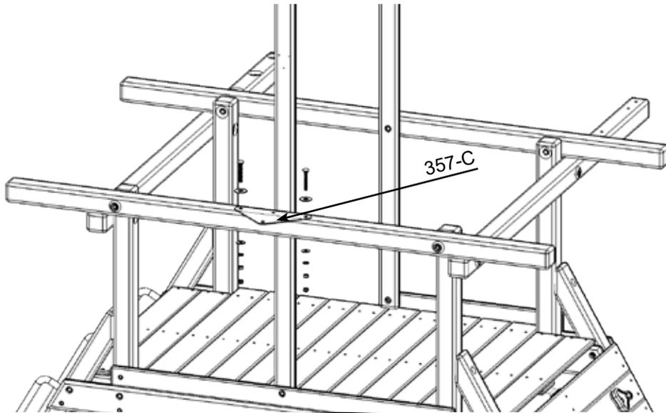
PLACE A-FRAME ON THE SB TOP JOIST AND SQUEEZE THE LEGS TOGETHER UNTIL LEVEL
