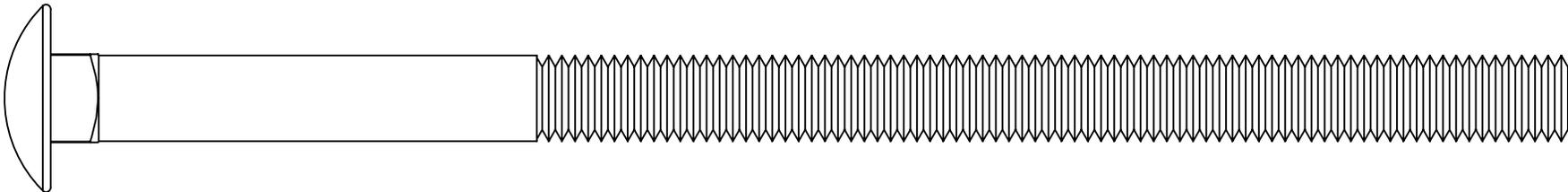
MEASUREMENT TAKEN FROM BOTTOM OF BOLT HEAD TO THE BOTTOM OF BOLT
