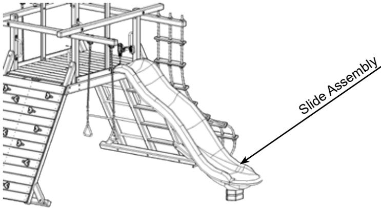
PLACE THE SLIDE ON THE DECK AND MARK HOLES TO BE DRILLED. THEN USING A 5/16" DRILL BIT, DRILL OUT THE MARKED LOCATIONS FOR THE HOLES. PLACE THE SLIDE BACK ON AND MOUNT AS SHOWN
