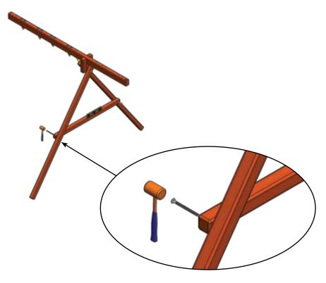
Above - Drill a 9/16" hole through the A-FRAME LEGS where your marks are. The holes should be slightly bigger than the bolt to allow for easy insert of the Carriage Bolt used.
