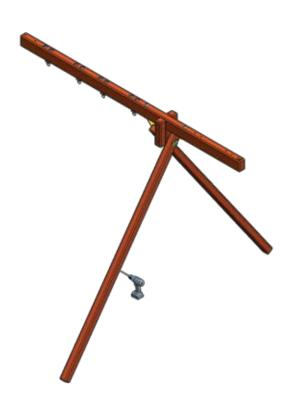
Above - Place the top corner of the A-FRAME CROSS-MEMBER to the outside of the A-FRAME LEG. Use a clamp or another person to hold one side while leveling. Once level and held down, use a 1/2" bolt of any size longer then 5" and a blunt object to mark a hole on the A-FRAME LEGS.
