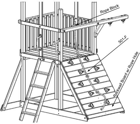
SLIP THE 501-F THROUGH THE ROPE BLOCK AND TIE A KNOT SECURING IT. TIE A COUPLE KNOTS AS YOU WORK YOUR WAY DOWN THE ROCKWALL. SLIP THE 501-F THROUGHT THE ROCKWALL BOARD W/ROPE HOLE AND TIE A KNOT OR 2 SECURING IT.
